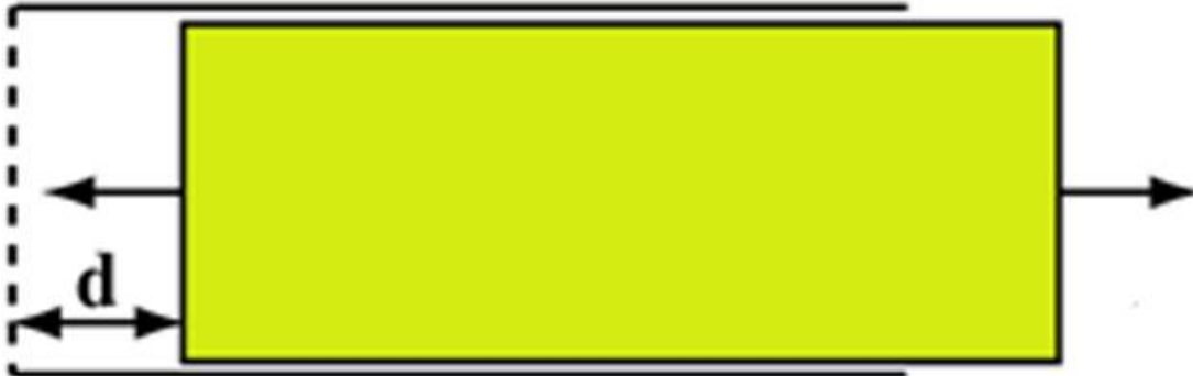
Fig. 2: Configuring Capacitive Position Sensor by Changing Dielectric Constant
