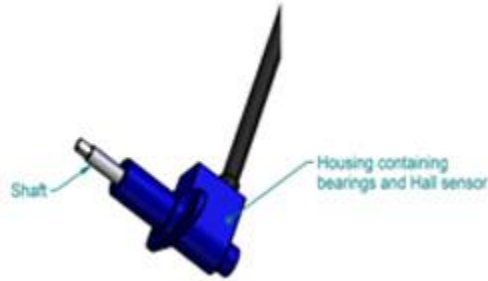
Fig. 13: Image Showing Hall Effect Based Magnetic Sensor
